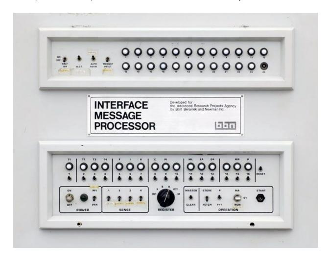
The Interface Message Processor (IMP) was the packet switching node used to interconnect participant networks to the ARPANET from the late 1960s to 1989. It was the first generation of gateways, which are known today as routers. An IMP required the connection to a host computer via a special bit-serial interface, The IMP software and the ARPA network
